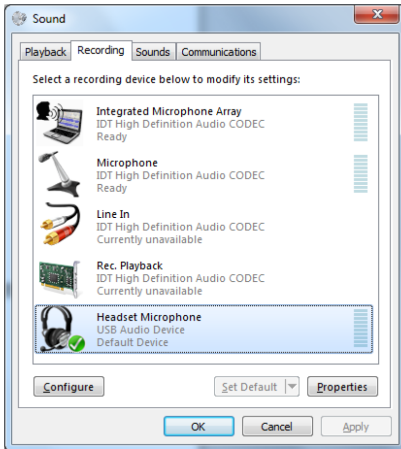
Figure 2 - Setting the headset as the default microphone
